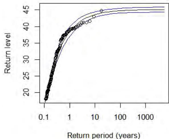
Return level plots in  $E_x$  (above) and  $E_y$  (top) for Nagycenk. Units for the return level are mV/km. 95% confidence limits are shown in blue. Circles denote measured data
