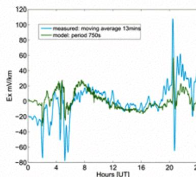
*Measured (blue) and modelled (green) geoelectric field at Eskdalemuir for the storm of 2<sup>nd</sup> October 2013. Differences are in part due to local induction effects. Electric field in the north direction is shown*
