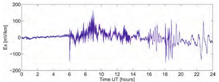
*Measured geo-electric field in mV/km at Eskdalemuir observatory, for a magnetically stormy day in 2013 (north component shown)*
