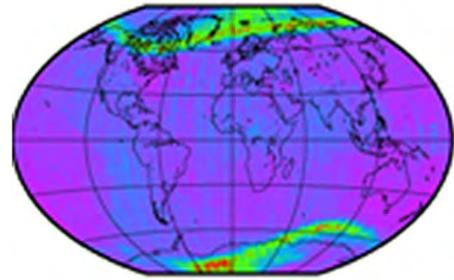
The two auroral zones are clearly identified (green/red) in this map of satellite magnetic measurements, where a model of the internal field has
