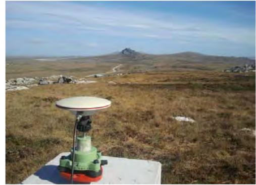
Surveying the new absolute observing pillar using differential GPS at Port Stanley Observatory, Falkland Islands
